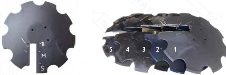
Figure 2: Test area and samples taken from the concave discs to be tested.
