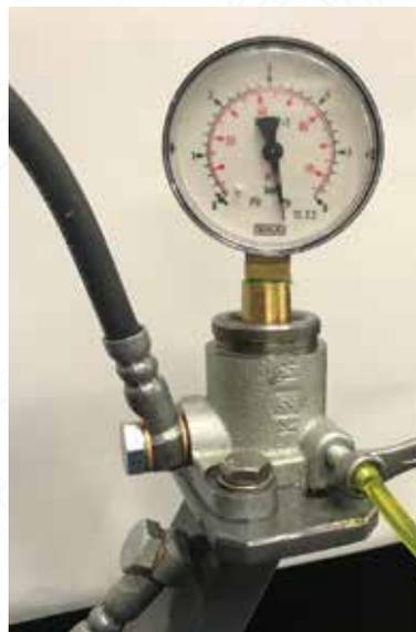
Figure 7 and 8: Possible pressure build-up before venting and after venting.
