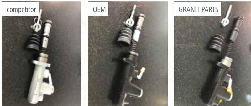
Figure 1: The master brake cylinders from the three suppliers. Dismantled MBC. Visual assessment and dimensional comparison of the installed components.
